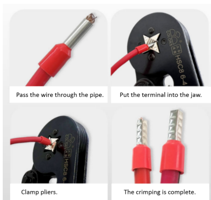
Figure 3-7 Crimping Cables
